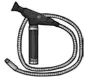
Fiber optic scopes can see around corners.
