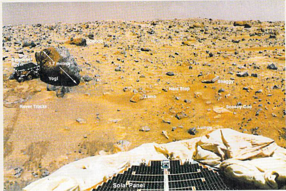
FIGURE 22.A Pathfinder 's rover Sojourner (left) obtaining data on the chemical composition of a Martian rock known as Yogi. (Photo courtesy of NASA)
